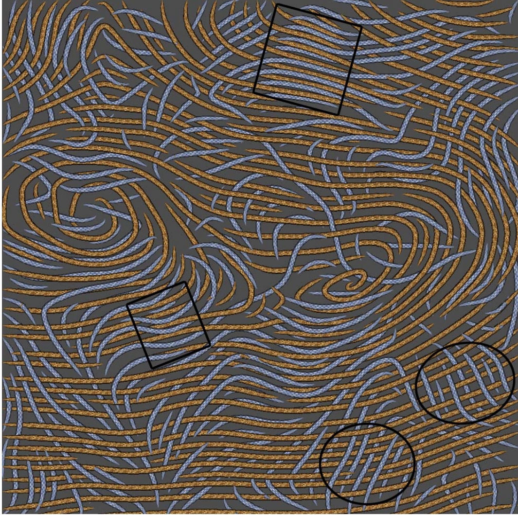
Figure 10. Visualization of multiple vector fields from a dual plane particle image velocimetry experiment. The tan texture mapped streamlines represent the velocity vector field. The light-blue textured streamlines represent the vorticity vector field. The regions within each rectangle depict areas where the vorticity field and the velocity field are parallel. The regions within each oval depict areas where the vorticity field and velocity field are orthogonal. The combination of vector fields within an image allows for a better understanding of the interactions between velocity and vorticity vector fields.
