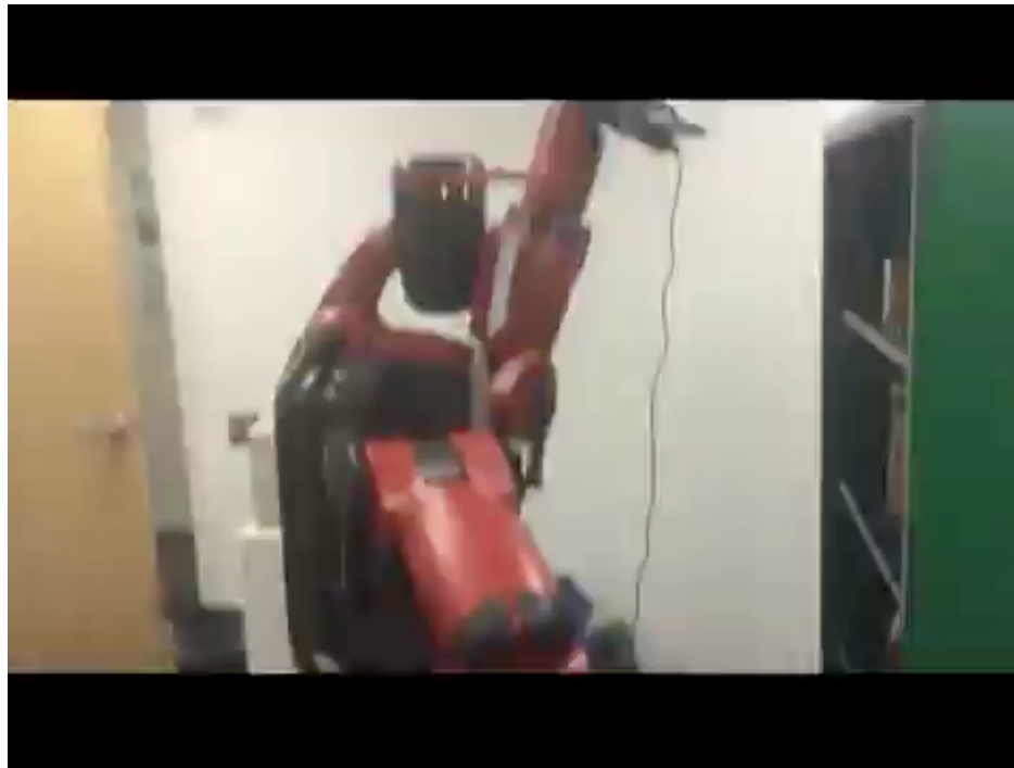
Baxter robot with a goal of fetching an specific object ie, Pringles from the shelf
