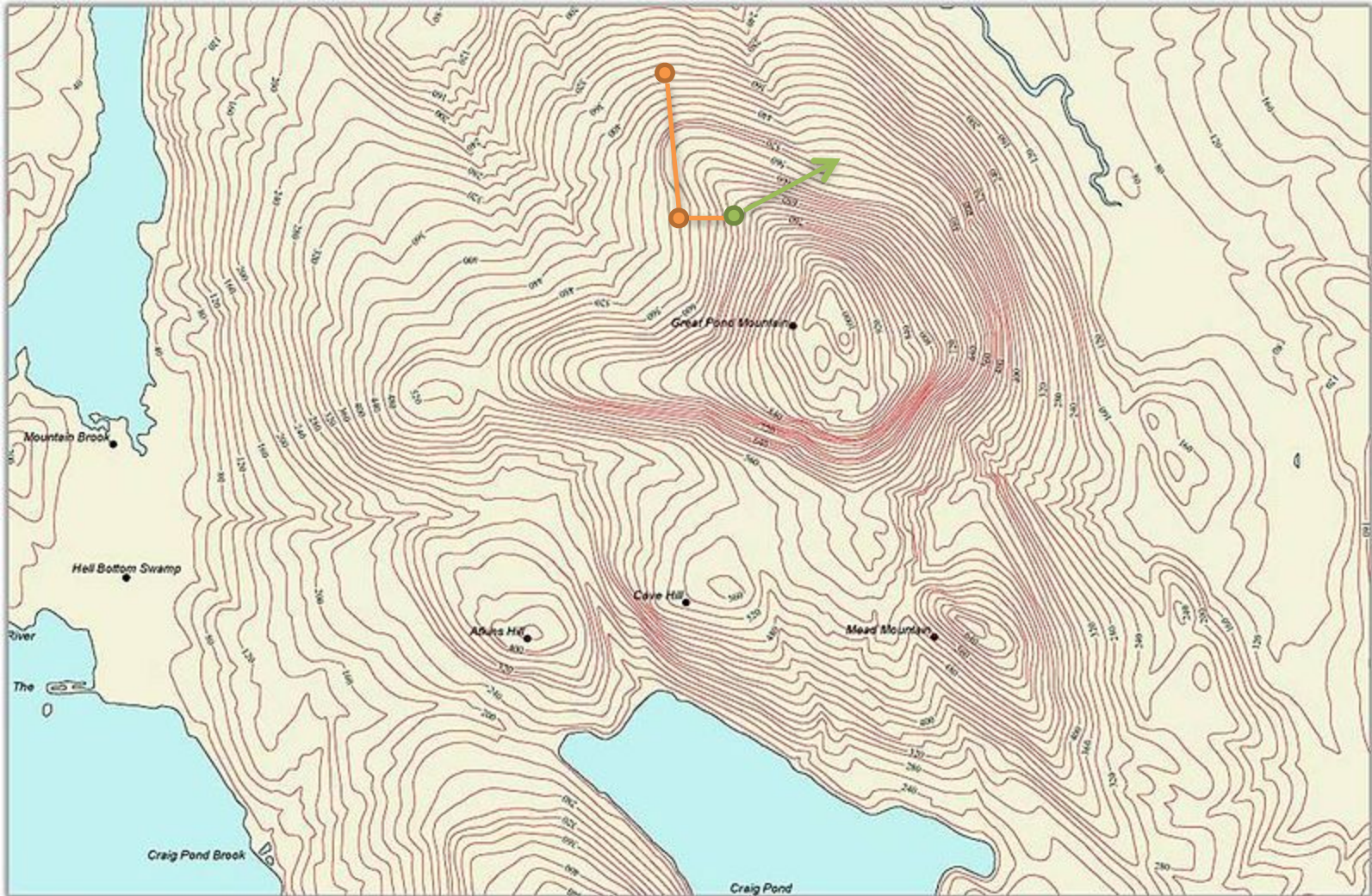
This visualization is called a contour map. It appears as if you are viewing a 3D surface from a bird's-eye perspective.
