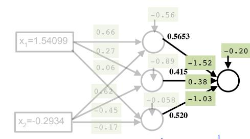
$$\mathbf{w^{T}_{X}} = \begin{bmatrix} w_{0} & w_{1} & w_{2} & w_{3} \end{bmatrix} \begin{bmatrix} -0.20 \\ 0.5653 \\ 0.415 \\ 0.520 \end{bmatrix} = \begin{bmatrix} 1 - 1.52 & 0.38 & -1.03 \end{bmatrix} \begin{bmatrix} -0.20 \\ 0.5653 \\ 0.415 \\ 0.520 \end{bmatrix} = 1 * (-0.20) + (-1.52) * 0.5653 + 0.38 * 0.415 + (-1.03) * (0.520) \end{bmatrix} = 1 * (-0.20) + (-1.52) * 0.5653 + 0.38 * 0.415 + (-1.03) * (0.520) \end{bmatrix} = 0.191$$
